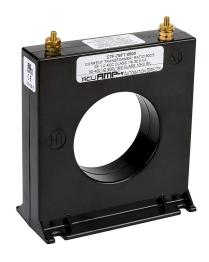
AcuAMP AC current transformer, solid core, 600A primary, 5A secondary, 2.5in diameter sensing window, 1% accuracy, M4 x 0.7 threaded terminal stud with nut.
