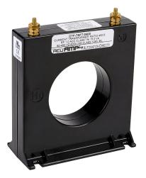
AcuAMP AC current transformer, solid core, 400A primary, 5A secondary, 2.5in diameter sensing window, 1% accuracy, M4 x 0.7 threaded terminal stud with nut.
