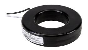
AcuAMP AC current transformer, solid core, 1000A primary, 5A secondary, 2.5in diameter sensing window, 1% accuracy, (2) 24in 16AWG lead wires.
