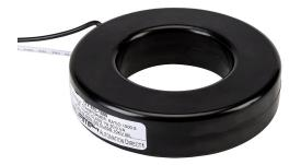
AcuAMP AC current transformer, solid core, 1000A primary, 5A secondary, 2.5in diameter sensing window, 1% accuracy, (2) 24in 16AWG lead wires.
