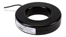
AcuAMP AC current transformer, solid core, 800A primary, 5A secondary, 2.5in diameter sensing window, 1% accuracy, (2) 24in 16AWG lead wires.
