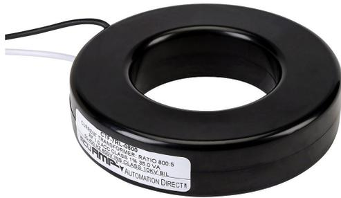
AcuAMP AC current transformer, solid core, 800A primary, 5A secondary, 2.5in diameter sensing window, 1% accuracy, (2) 24in 16AWG lead wires.
