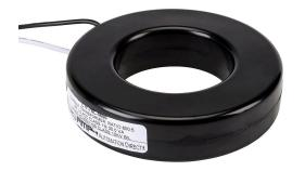
AcuAMP AC current transformer, solid core, 600A primary, 5A secondary, 2.5in diameter sensing window, 1% accuracy, (2) 24in 16AWG lead wires.
