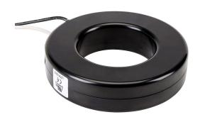
AcuAMP AC current transformer, solid core, 400A primary, 5A secondary, 2.5in diameter sensing window, 1% accuracy, (2) 24in 16AWG lead wires.
