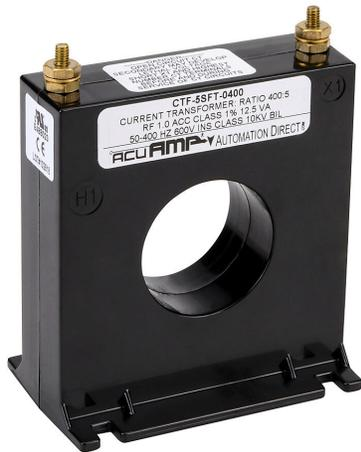
AcuAMP AC current transformer, solid core, 400A primary, 5A secondary, 1.56in diameter sensing window, 1% accuracy, M4 x 0.7 threaded terminal stud with nut.
