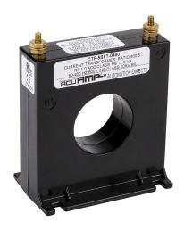
AcuAMP AC current transformer, solid core, 400A primary, 5A secondary, 1.56in diameter sensing window, 1% accuracy, M4  $\times$  0.7 threaded terminal stud with nut.
