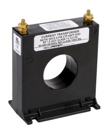
AcuAMP AC current transformer, solid core, 200A primary, 5A secondary, 1.56in diameter sensing window, 1% accuracy, M4 x 0.7 threaded terminal stud with nut.
