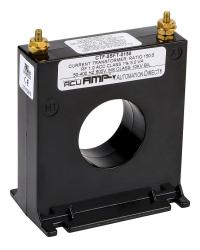
AcuAMP AC current transformer, solid core, 150A primary, 5A secondary, 1.56in diameter sensing window, 1% accuracy, M4 x 0.7 threaded terminal stud with nut.
