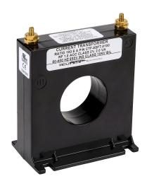
AcuAMP AC current transformer, solid core, 100A primary, 5A secondary, 1.56in diameter sensing window, 2% accuracy, M4 x 0.7 threaded terminal stud with nut.
