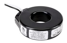
AcuAMP AC current transformer, solid core, 200A primary, 5A secondary, 1.56in diameter sensing window, 1% accuracy, (2) 24in 16AWG lead wires.
