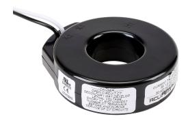
AcuAMP AC current transformer, solid core, 200A primary, 5A secondary, 1.56in diameter sensing window, 1% accuracy, (2) 24in 16AWG lead wires.
