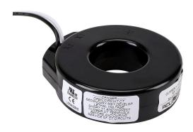
AcuAMP AC current transformer, solid core, 150A primary, 5A secondary, 1.56in diameter sensing window, 1% accuracy, (2) 24in 16AWG lead wires.
