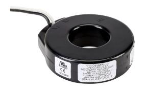
AcuAMP AC current transformer, solid core, 100A primary, 5A secondary, 1.56in diameter sensing window, 2% accuracy, (2) 24in 16AWG lead wires.
