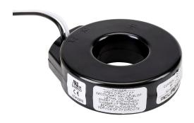
AcuAMP AC current transformer, solid core, 50A primary, 5A secondary, 1.56in diameter sensing window, 2% accuracy, (2) 24in 16AWG lead wires.
