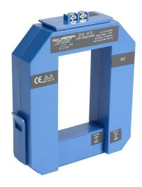
AcuAMP AC current transformer, split core, 1000A primary, 5A secondary, 2.36 x 3.49in sensing window, 1% accuracy, screw terminal.
