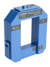
AcuAMP AC current transformer, split core, 800A primary, 5A secondary,  $2.36 \times 3.49$ in sensing window, 1% accuracy, screw terminal.
