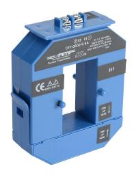
AcuAMP AC current transformer, split core, 600A primary, 5A secondary,  $1.19 \times 2.22$ in sensing window, 1% accuracy, screw terminal.
