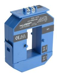
AcuAMP AC current transformer, split core, 400A primary, 5A secondary,  $1.19 \times 2.22$ in sensing window, 1% accuracy, screw terminal.
