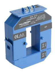
AcuAMP AC current transformer, split core, 200A primary, 5A secondary, 1.19 x 2.22in sensing window, 1% accuracy, screw terminal.
