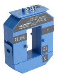
AcuAMP AC current transformer, split core, 150A primary, 5A secondary, 1.19 x 2.22in sensing window, 1.5% accuracy, screw terminal.
