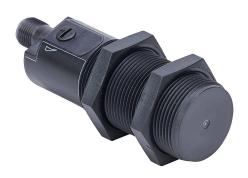
AutomationDirect capacitive proximity sensor, tubular, 30mm diameter x 92mm body, polybutylene terephthalate housing, PNP, N.C. output, 25mm sensing distance, non-flush, 40 Hz switching frequency, IP65 IP67 IP69K, 4-pin M12 quick-disconnect.
