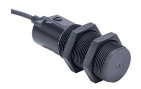
AutomationDirect capacitive proximity sensor, tubular, 30mm diameter x 92mm body, polybutylene terephthalate housing, PNP, N.C. output, 25mm sensing distance, non-flush, 40 Hz switching frequency, IP65 IP67 IP69K, pigtail.
