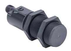
AutomationDirect capacitive proximity sensor, tubular, 30mm diameter x 92mm body, polybutylene terephthalate housing, PNP, N.C. output, 15mm sensing distance, flush, 40 Hz switching frequency, IP65 IP67 IP69K, 4-pin M12 quick-disconnect.
