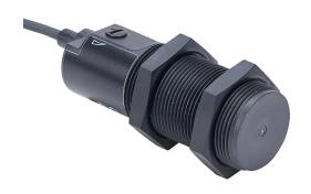
AutomationDirect capacitive proximity sensor, tubular, 30mm diameter x 92mm body, polybutylene terephthalate housing, PNP, N.C. output, 15mm sensing distance, flush, 40 Hz switching frequency, IP65 IP67 IP69K, pigtail.
