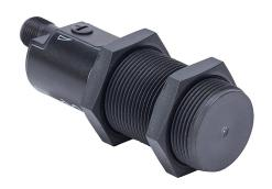
AutomationDirect capacitive proximity sensor, tubular, 30mm diameter x 92mm body, polybutylene terephthalate housing, NPN, N.C. output, 25mm sensing distance, non-flush, 40 Hz switching frequency, IP65 IP67 IP69K, 4-pin M12 quick-disconnect.
