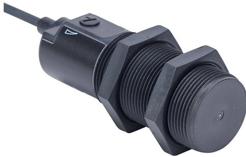
AutomationDirect capacitive proximity sensor, tubular, 30mm diameter x 92mm body, polybutylene terephthalate housing, NPN, N.C. output, 25mm sensing distance, non-flush, 40 Hz switching frequency, IP65 IP67 IP69K, pigtail.
