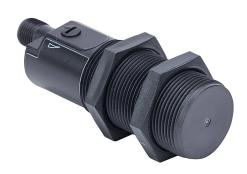
AutomationDirect capacitive proximity sensor, tubular, 30mm diameter x 92mm body, polybutylene terephthalate housing, PNP, N.O. output, 25mm sensing distance, non-flush, 40 Hz switching frequency, IP65 IP67 IP69K, 4-pin M12 quick-disconnect.
