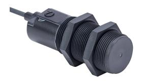
AutomationDirect capacitive proximity sensor, tubular, 30mm diameter x 92mm body, polybutylene terephthalate housing, PNP, N.O. output, 25mm sensing distance, non-flush, 40 Hz switching frequency, IP65 IP67 IP69K, pigtail.
