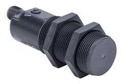
AutomationDirect capacitive proximity sensor, tubular, 30mm diameter x 92mm body, polybutylene terephthalate housing, PNP, N.O. output, 15mm sensing distance, flush, 40 Hz switching frequency, IP65 IP67 IP69K, 4-pin M12 quick-disconnect.
