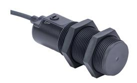
AutomationDirect capacitive proximity sensor, tubular, 30mm diameter x 92mm body, polybutylene terephthalate housing, PNP, N.O. output, 15mm sensing distance, flush, 40 Hz switching frequency, IP65 IP67 IP69K, pigtail.
