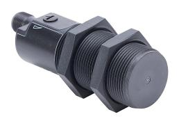
AutomationDirect capacitive proximity sensor, tubular, 30mm diameter x 92mm body, polybutylene terephthalate housing, NPN, N.O. output, 25mm sensing distance, non-flush, 40 Hz switching frequency, IP65 IP67 IP69K, 4-pin M12 quick-disconnect.
