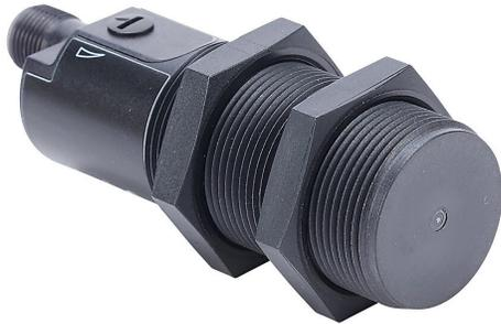
AutomationDirect capacitive proximity sensor, tubular, 30mm diameter x 92mm body, polybutylene terephthalate housing, NPN, N.O. output, 25mm sensing distance, non-flush, 40 Hz switching frequency, IP65 IP67 IP69K, 4-pin M12 quick-disconnect.
