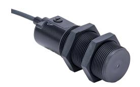
AutomationDirect capacitive proximity sensor, tubular, 30mm diameter x 92mm body, polybutylene terephthalate housing, NPN, N.O. output, 25mm sensing distance, non-flush, 40 Hz switching frequency, IP65 IP67 IP69K, pigtail.
