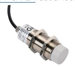
Micro Detectors capacitive proximity sensor, tubular, 30mm diameter x 71mm body, nickel-plated brass housing, NPN, N.C. output, 20mm sensing distance, non-flush, 100 Hz switching frequency, IP65, pigtail.
