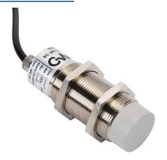
Micro Detectors capacitive proximity sensor, tubular, 30mm diameter x 71mm body, nickel-plated brass housing, PNP, N.O. output, 20mm sensing distance, non-flush, 100 Hz switching frequency, IP65, pigtail.
