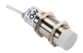
Micro Detectors capacitive proximity sensor, tubular, 30mm diameter x 71mm body, nickel-plated brass housing, NPN, N.O. output, 20mm sensing distance, non-flush, 100 Hz switching frequency, IP65, pigtail.
