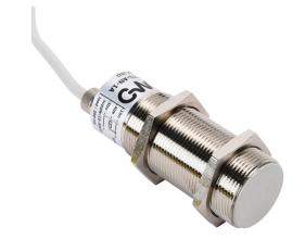
Micro Detectors capacitive proximity sensor, tubular, 30mm diameter x 71mm body, nickel-plated brass housing, NPN, N.O. output, 15mm sensing distance, flush, 100 Hz switching frequency, IP65, pigtail.
