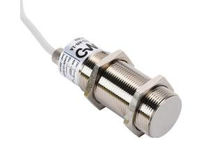
Micro Detectors capacitive proximity sensor, tubular, 30mm diameter x 71mm body, nickel-plated brass housing, NPN, N.O. output, 15mm sensing distance, flush, 100 Hz switching frequency, IP65, pigtail.
