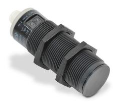
AutomationDirect capacitive proximity sensor, tubular, 30mm diameter x 90mm body, polybutylene terephthalate housing, NPN/PNP, N.O./N.C. selectable output, 40mm sensing distance, non-flush, 10 Hz switching frequency, IP65 IP67, 4-pin M12 quick-disconnect.
