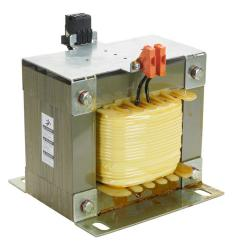
BLOCK control transformer, open core, 2.5 kVA, 1-phase, 600 VAC, 120 VAC secondary, 50/60 Hz, panel mount.
