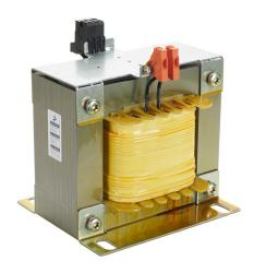
BLOCK control transformer, open core, 2 kVA, 1-phase, 600 VAC, 120 VAC secondary, 50/60 Hz, panel mount.
