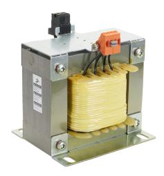
BLOCK control transformer, open core, 2 kVA, 1-phase, 240/480 VAC, 120 VAC secondary, 50/60 Hz, panel mount.
