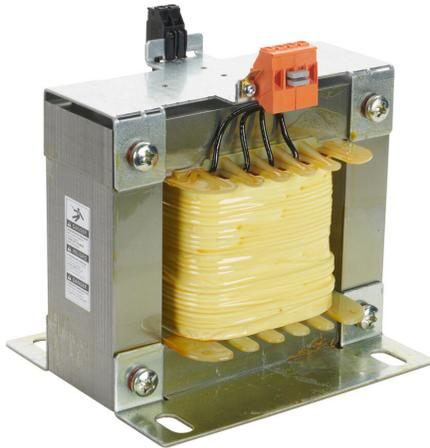
BLOCK control transformer, open core, 1.5 kVA, 1-phase, 240/480 VAC, 120 VAC secondary, 50/60 Hz, panel mount.
