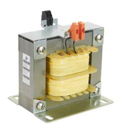
BLOCK control transformer, open core, 1 kVA, 1-phase, 600 VAC, 120 VAC secondary, 50/60 Hz, panel mount.
