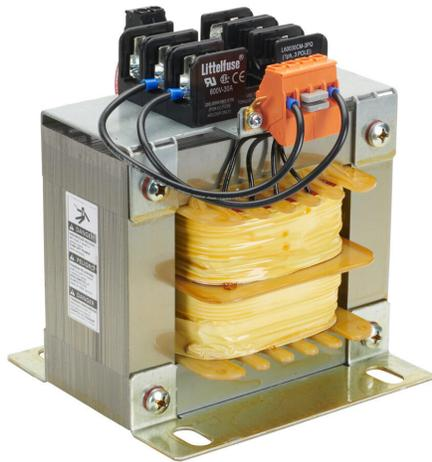
BLOCK control transformer, open core, 750 VA, 1-phase, 240/480 VAC, 120 VAC secondary, 50/60 Hz, fused, panel mount.
