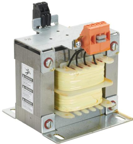
BLOCK control transformer, open core, 350 VA, 1-phase, 240/480 VAC, 120 VAC secondary, 50/60 Hz, panel mount.
