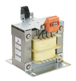
BLOCK control transformer, open core, 350 VA, 1-phase, 240/480 VAC, 120 VAC secondary, 50/60 Hz, panel mount.
