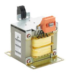
BLOCK control transformer, open core, 250 VA, 1-phase, 600 VAC, 24 VAC secondary, 50/60 Hz, panel mount.
