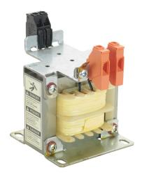
BLOCK control transformer, open core, 75 VA, 1-phase, 600 VAC, 24 VAC secondary, 50/60 Hz, panel mount.
