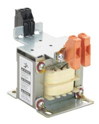
BLOCK control transformer, open core, 50 VA, 1-phase, 600 VAC, 24 VAC secondary, 50/60 Hz, panel mount.
