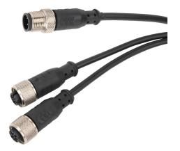
ReeR muting emitter cable, 5-pin M12 quick-disconnect to (2) 5-pin M12 quick-disconnects, 5-pole, 24 VDC, PVC jacket, black, unshielded, 1.3ft/400mm cable length, IP67.
