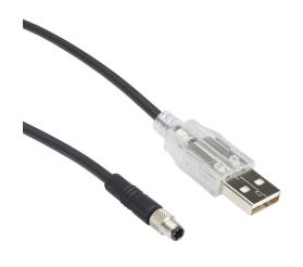
ReeR programming cable, USB Type A male to M5, black, 6.5ft/2m cable length. For use with Micron X-AC analog models.
