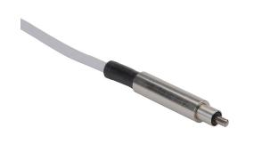
Metrol limit switch, precision touch, 6mm diameter, smooth, 42mm length, 1.5mm radius head, stainless steel, 2mm plunger, 1N contact force, (1) N.O. contact(s), 9.8ft/3m cable length, pigtail.
